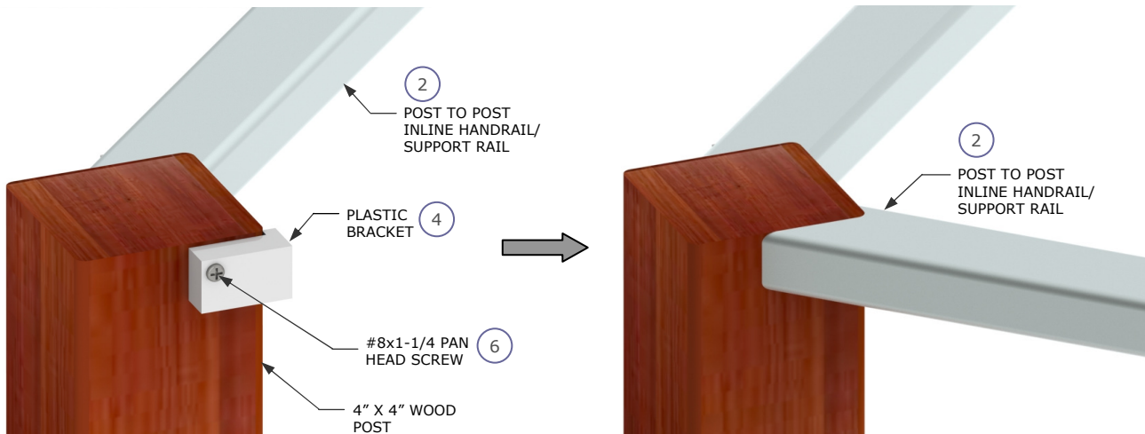
Fig 16: 90deg Post-to-Post Instructions
